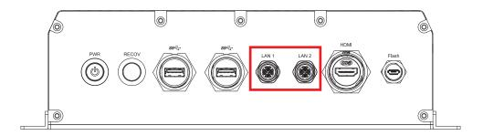
There are two LAN ports supporting 10/100/1000 Mbps Ethernet connections on the front side of RAC-1000/1100 series.
