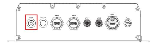
The Power Button is a non-latched switch with LED indication.
