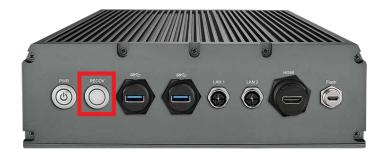
**Step 3** While holding the "RECOV" button, power on the system. Continue to hold the "RECOV" button for two seconds, and release.
