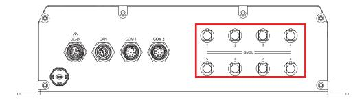
There are eight FAKRA connectors in the rear side of RAC-1000. Each camera connects to the RAC-1000 through a single coax cable. Using GMSL2 (Gigabit Multimedia Serial Link) connections, the cameras are connected to a two-port deserializer. The output of the deserializer is MIPI CSI-2.
