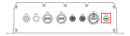
The RAC-1000/1100 USB Recovery mode provides an alternate boot device (USB). In this mode, the system is connected to a host system and boots over USB. This is used when a new image needs to be flashed. USB0 must be available to use as USB Device for USB Recovery Mode.
