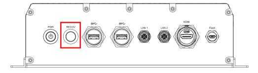
Used to enter Force Recovery Mode. Button is held down while either system is first powered on, or by pressing & releasing reset button while Recovery button is pressed.
