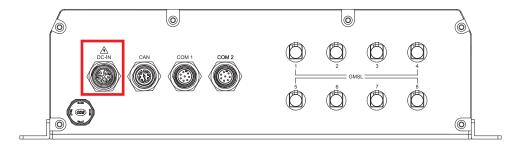
RAC-1000/RAC-1100 series supports 9V to 50V DC wide range power input by DC-IN connector in the rear side.
