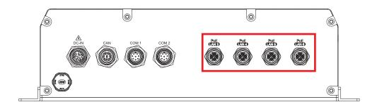
There are 4 LAN connectors in the rear side of RAC-1100. It supports IEEE 802.3at (PoE+) Power over Ethernet (PoE) connection delivering up to 25W/54V per port and 1000BASE-T gigabit data signals over standard Ethernet Cat 5/Cat 6 cable.
