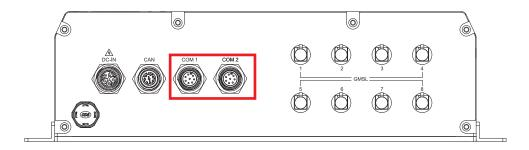
The COM 1, 2 can be configured for RS-232, RS-422, or RS-485 with auto flow control communication. The default definition of COM 1 and COM2 is RS-232; if you want to use RS-422 or RS-485, you must select the desired COM mode through GPIO.
