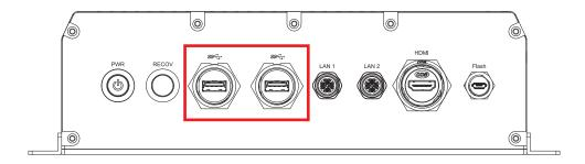
There are 2 USB 3.2 Gen1 connections available supporting up to 5Gb per second data rate in the front panel of RAC-1000/1100 series. It is also compliant with the requirements of Speed (SS), High Speed (HS), Full Speed (FS) and Low Speed (LS).
