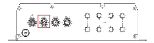
RAC-1000/RAC-1100 series supports CAN Bus by CAN connector in the rear side. The pin define of CAN 1 & CAN 2 are listed as follows:
